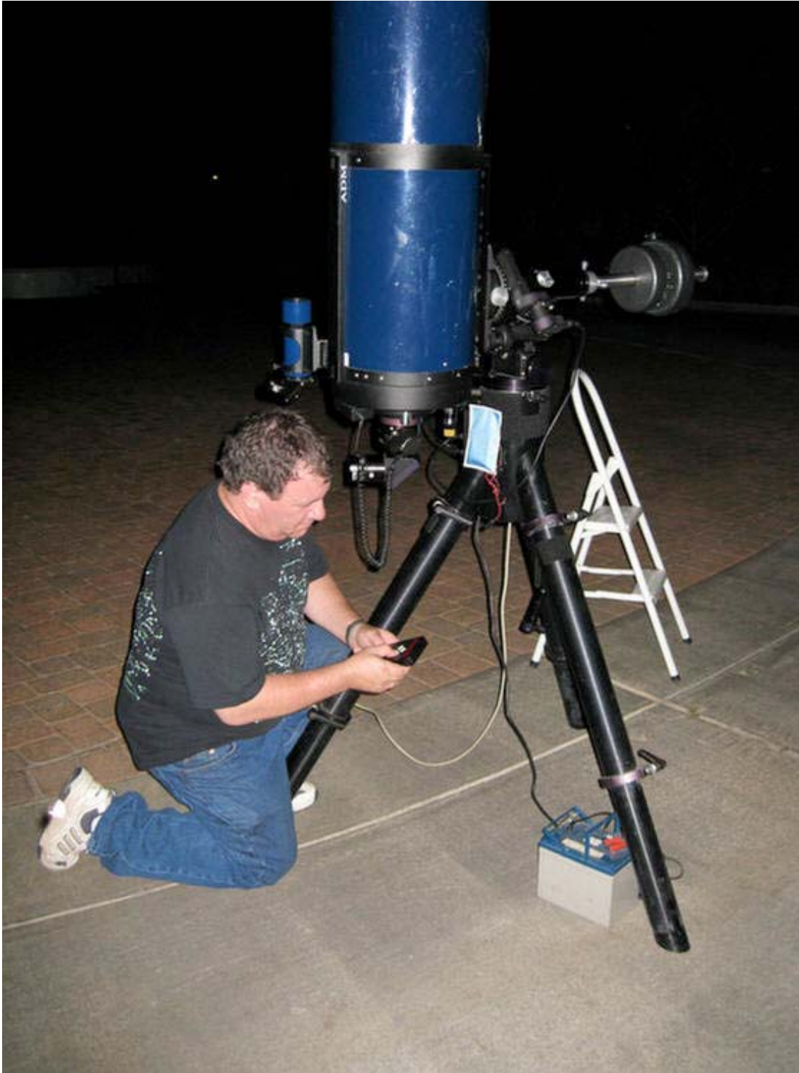
Checking alignment; the hand held device controls the telescope!
