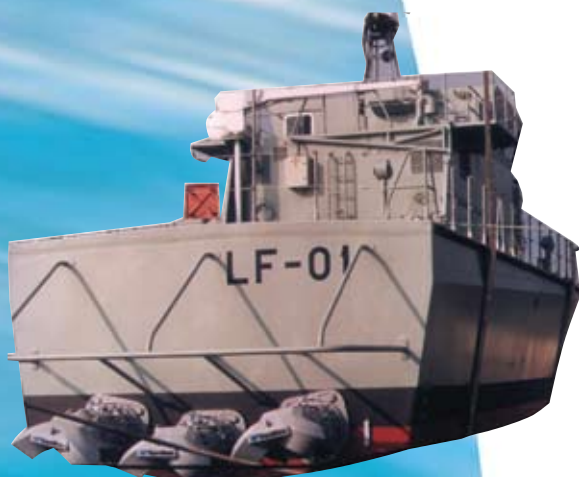
Triple HM521 Waterjets in a 20m Patrol Craft.
